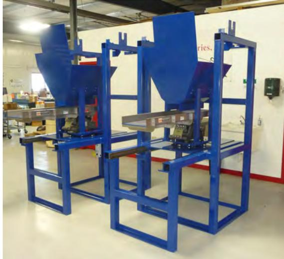
These plating line unloaders were custom built for the automation of a plating line.
